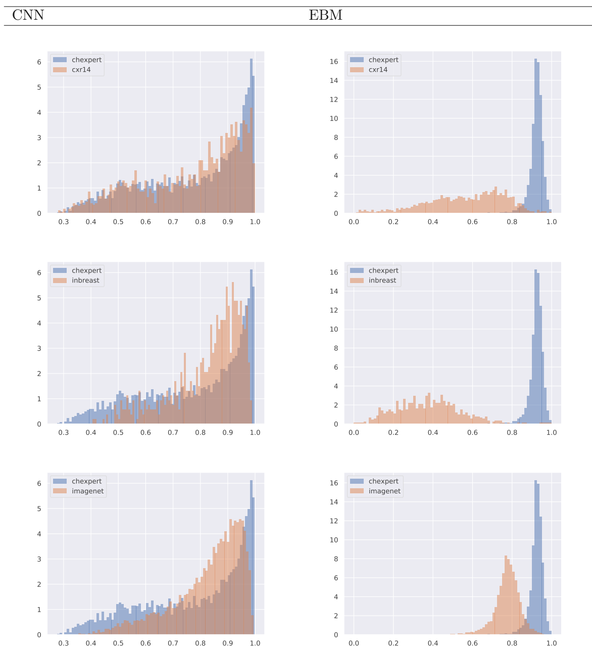
Figure 7.5: Visualisation of score distributions from the pre-trained DL model and the EBM. The first row shows the distributions of softmax (DL model) and energy-based (EBM model) probabilities between the CheXpert dataset and the CXR14 dataset; the second row the the distributions between the CheXpert dataset and the InBreast dataset and the third the distributions between the CheXpert dataset and the ImageNet dataset. The bottom row shows the distribution probabilities from the energy model between the CheXpert dataset and the out of distribution datasets. The degree of overlap is indicative of how well the respective model can find fake data. The x-axis is the score, softmax or energy, and the y-axis in the frequency
