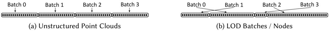
Fig. 3. (a) For unstructured, Morton-code-ordered data sets, we group 10 240 consecutive points into a batch. (b) For hierarchical (LOD) data, each node refers to a batch of variable size, potentially out of order.
