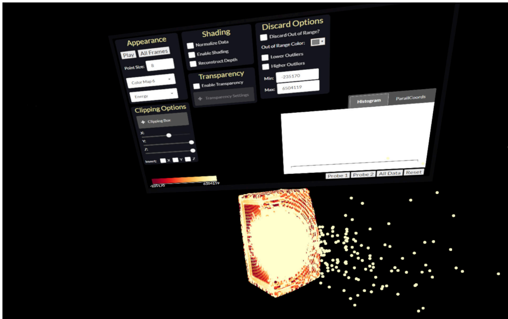
(b) Using the axis aligned clipping planes from the C lipping panel to cut the visualization in X and Y directions
