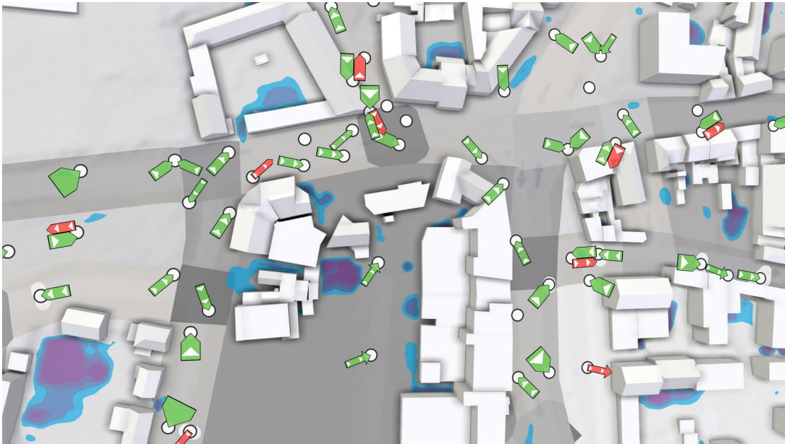
Figure 3.14: Glyphs show details about the sewer-surface coupling.
