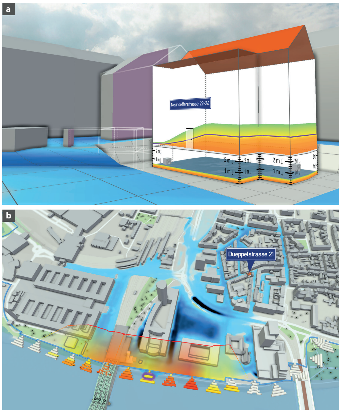
Figure 2.1: Understanding the uncertain vulnerability of a selected building to a multitude of flooding scenarios. (a) Adverse impact on a selected building, including cellar flooding. The probability of water reaching a particular level varies around the building and is mapped onto the façades. (b) Vulnerability of the building to floodwall breaches, shown along the floodwall.
