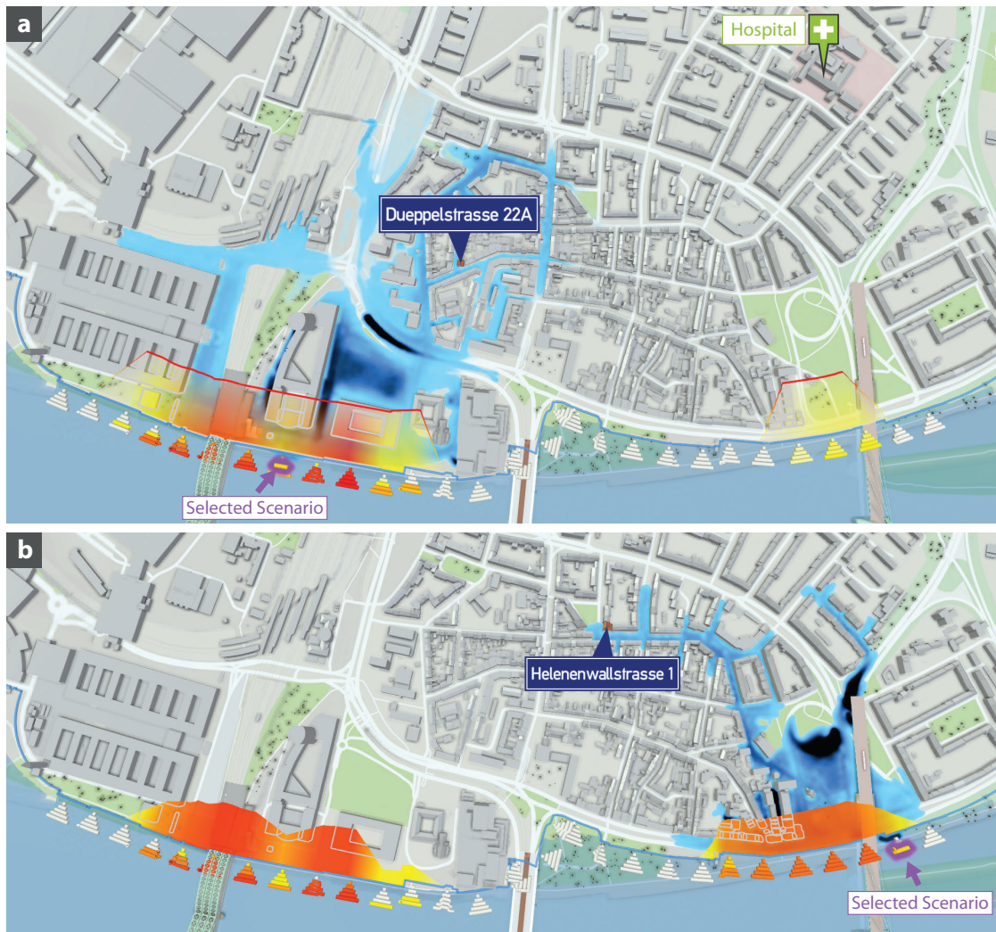
Figure 2.9: Floodwall breach scenario selection. (a) Vulnerability with respect to the hospital accessibility. A scenario is selected by clicking on a width bar, showing the aggregated water depths on the terrain. (b) Non-expert view of vulnerability with respect to the damage of the building of interest. The worst-case values are shown in the plot and width bars. The worst-case water depths are displayed for the selected scenario.
