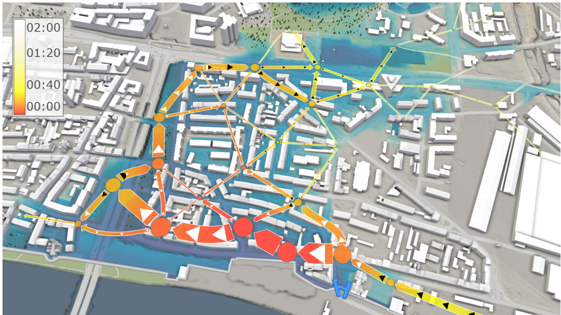
Figure 3.9: Overlay visualization of wave arrival times [hh:mm] after a floodwall breach.
