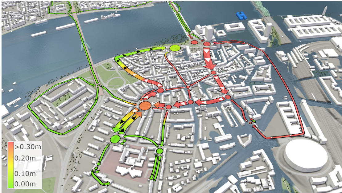
Figure 3.8: Overlay visualization of road inaccessibility due to inundation.
