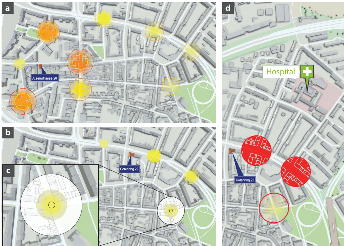
Figure 2.6: Vulnerability to sewer overflows, presented for experts. (a) Sewer locations potentially dangerous for the selected building. (b) For another building, different locations are dangerous. (c) On mouse-over, a context legend is displayed, showing the 0 % and 100 % bounds. The building contours preserve the spatial context. (d) Vulnerability with respect to the accessibility of the nearest hospital.
