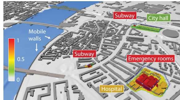
Figure 2: Area of interest protected by mobile walls. If overtopping happens, vital infrastructure should be kept water-free. The importance of objects is outlined by user sketches, coloring buildings and areas according to user-defined priorities between 0 and 1.
