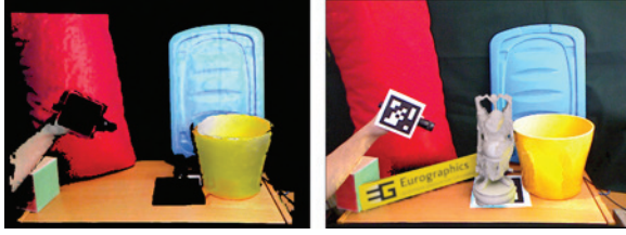
Figure 7: The left image shows a simple Phong rendering with the VPLs used for BRDF estimation. In the right image a virtual pocket lamp illuminates the real scene. Note the yellow color bleeding on the real desk and on the virtual Buddha.
