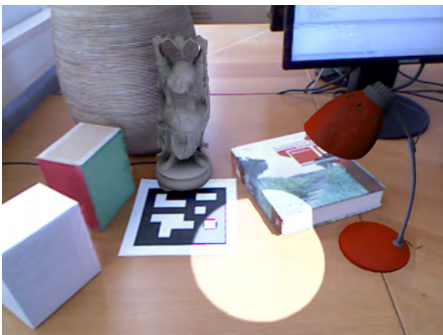
Figure 1: This figure shows a mixed reality scenario where a virtual table lamp illuminates the real and virtual objects causing indirect shadows from the Buddha on a real vase. The scene is reconstructed during run-time and rendered at 17.5 fps.
