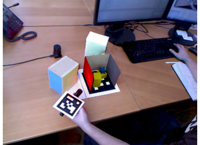
Figure 12: The real pocket lamp illuminates the virtual Cornell Box and causes red color bleeding on the desk and the real box.
