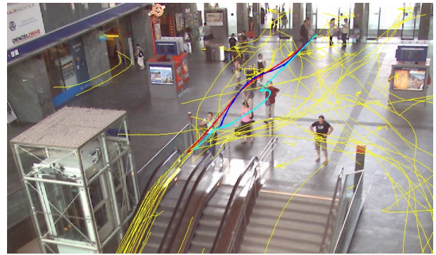
Fig. 6. Simulation validation. In a set of real trajectories, one real trajectory (in red) is replaced by a simulated trajectory (light blue and dark blue, see text).
