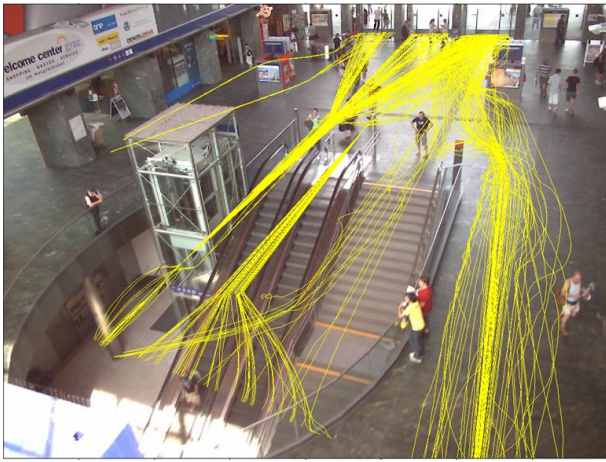
Fig. 5. Simulated trajectories, with original destination flow obtained from data visualized in Fig. 4.
