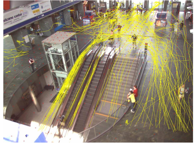
Fig. 4. All smoothed trajectories with more than 30 trajectory states, computed from a 15 minutes video.
