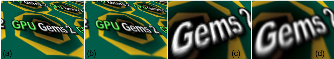
Figure 3. Comparing Texture-Filter Quality with Bilinear and Bicubic Reconstruction Filters (a, c) Bilinear and (b, d) bicubic reconstruction filters.
