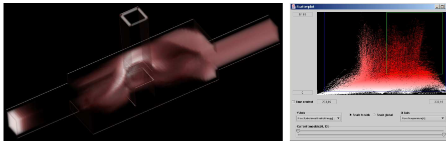
Fig. 9. Visualization of flow through a T-junction. The visualization focuses on a flow subset which is characterized by high temperature and high turbulent kinetic energy. The junction-geometry is added as context (contour rendering).
