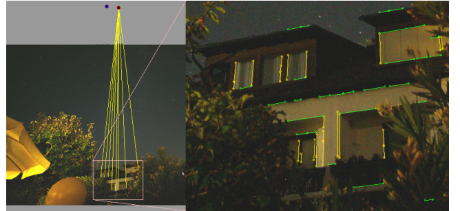
Figure 5: The vertical vanishing point is calculated using the extracted vertical lines of the house (zoomed out). It serves as reference value for the determined zenith direction which intersects the image plane at the position indicated by the left dot.
