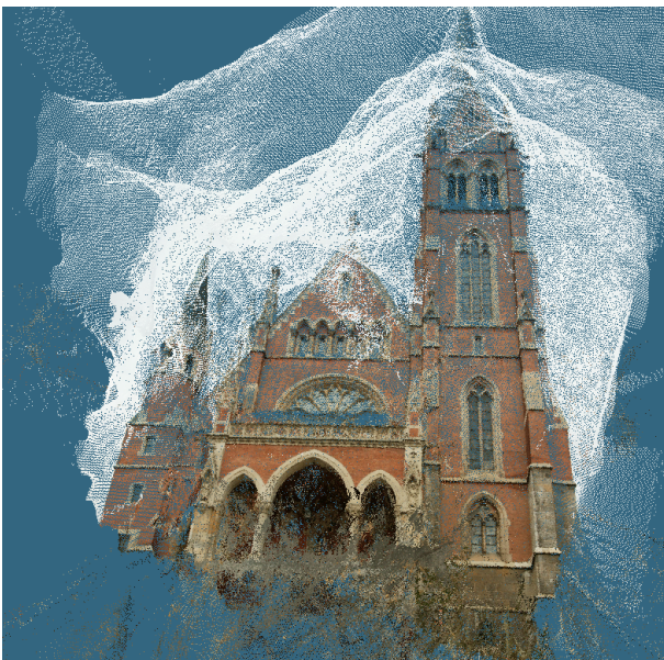
Figure 2: 3D point cloud from of the Herz-Jesu church in Graz. The generated 3D point cloud includes many outliers from areas like the sky, thus a segmentation and interpretation of the scene is needed.
