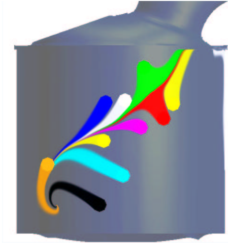
Figure 10: Dye injection is used to highlight areas of the flow in combination on the boundary surface of an intake port and combustion chamber.
