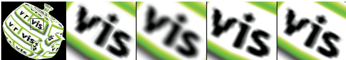
Figure 2: Surface textured teapot using tent, cubic B-spline, Catmull-Rom spline and Kaiser windowed sinc filters (from left to right).
